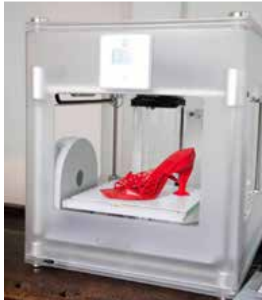
Three-dimensional (3D) printers gradually lay a variety of materials from plastic to human cells one on top of another to form shapes and produce materials like shoes, jewelry, furniture and cars. 3D printers are now making parts of a human body like skin and knees.
