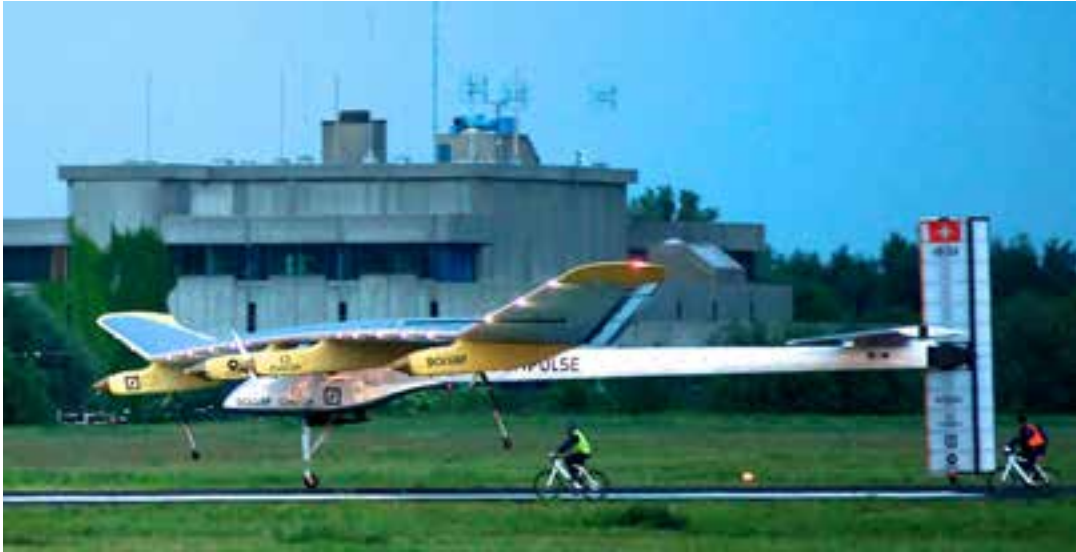
Solar Impulse, an electric aircraft circumnavigating the globe in 2016-17, is a single-seat plane powered by solar cells and capable of taking off under its own power. The design allows the aircraft to remain airborne for several days. Solar Impulse 2 was converted for unmanned flights to "run applications" that cannot currently be performed by satellites for communication, measurements and observations for agriculture, infrastructure planning and other purposes.
