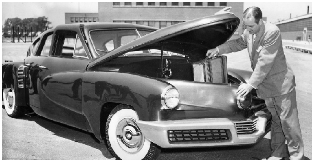
Preston Tucker places luggage in the trunk of his Tucker 48 . As you can see, the trunk was located in the front of the car while the engine was located in the rear of the Tucker 48 !
