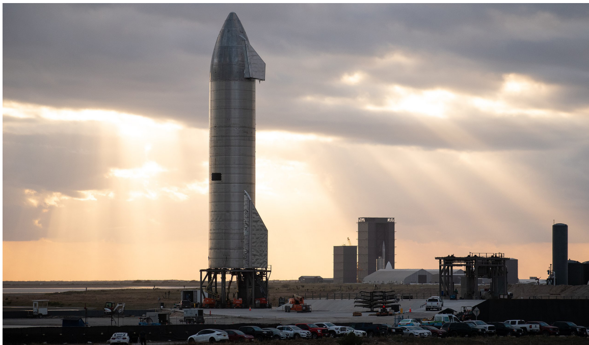
photograph of the SPACE X Starship X rocket. SpaceX was founded in 2002 by Elon Musk, with the goal of reducing space transportation costs to enable the colonization of Mars Starship is a fully-REUSABLE, super-heavy-lift launch vehicle. Starship is a two-stage-to-orbit launch vehicle, consisting of the Super Heavy booster stage and the Starship second stage or spacecraft. The spacecraft has four main variants: cargo, crew, propellant tanker, and lunar lander. Starship rockets are designed for rapid reuse after a vertical landing. Starship rockets use liquid oxygen plus liquid methane for fuel and are powered by Raptor engines. Once in orbit, the Starship rockets can be refueled by Starship fuel tankers to get them to higher orbits or destinations in the inner Solar System.
